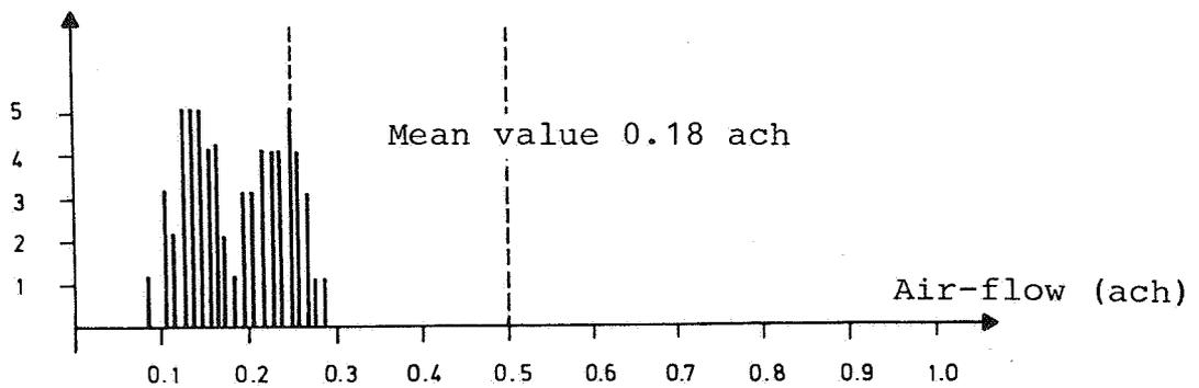
Figure 2B. Measured air-flow through the ventilation system (ach)
