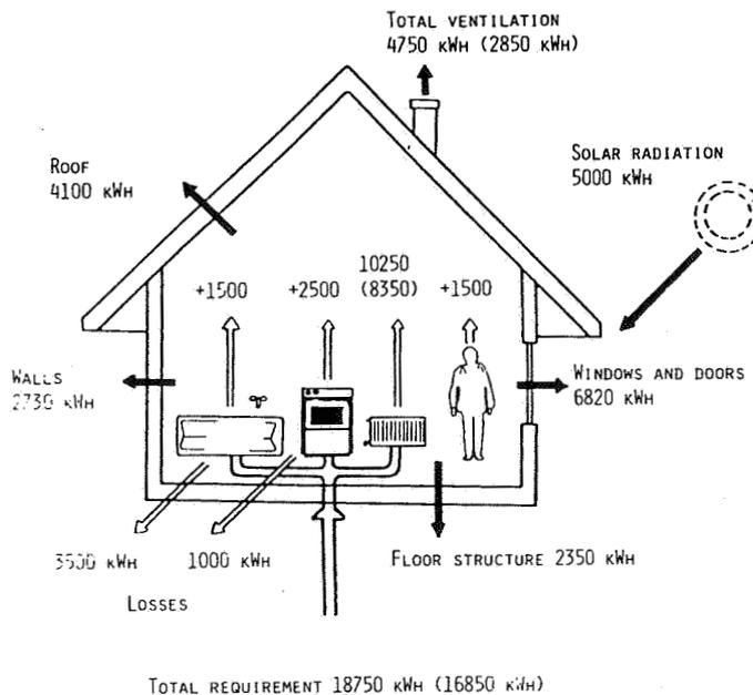
Figure 1. Heat balance at a total ventilation of 0.3 and 0.5 changes per hour. The values within parentheses correspond to 0.3 ach.
