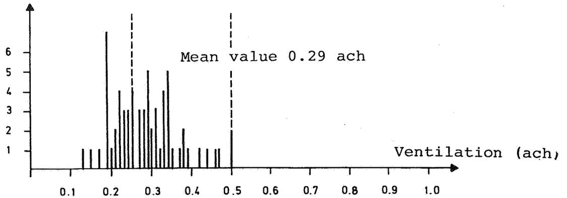
Figure 2A. Measured total ventilation (ach).
