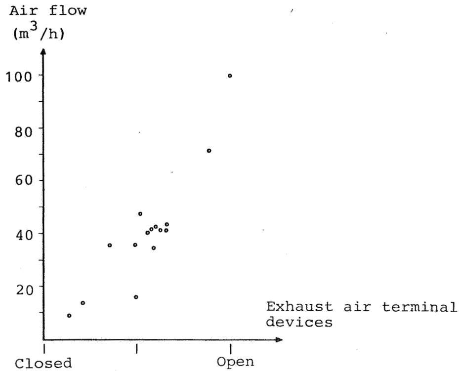
Figure 3. Recorded air-flow and adjustment of exhaust air terminal devices. The devices were presumed to have an air-flow of 50 m<sup>3</sup>/h
