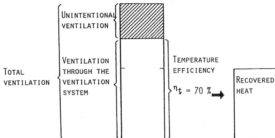
Figure 4. The limitation of the temperature efficiency
