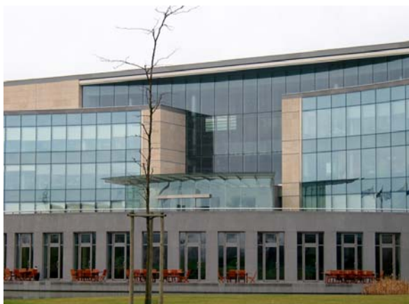
Fig. 34: Airtight outdoor façade (cannot be opened even not for maintenance reasons) UCB Center (Brussels)
