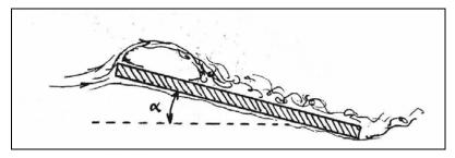
Figure 10 Flow separation on the leading edge of a flat plate in incidence
