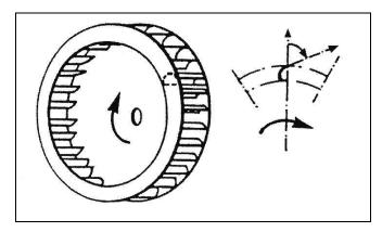
Figure 6 Centrifugal impeller with forward-curved blades
