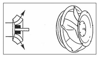
Figure 7 Impeller of a mixed flow fan
