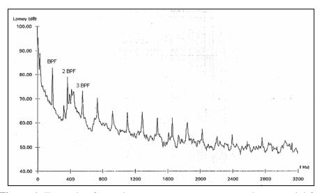
Figure 1 Example of sound pressure spectrum measured on an axial fan
