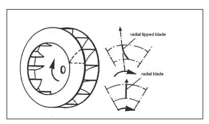
Figure 5 Centrifugal impeller with radial blades
