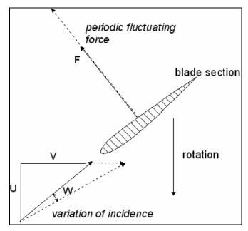
**Figure 9** Velocity triangle at the blade leading edge
