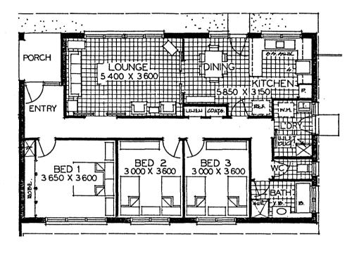
Figure 2 Plan of the dwelling used for the example contained in Appendix B.
