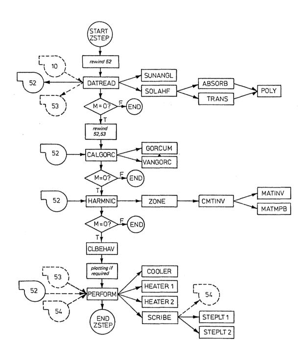
Figure 1 Logical structure for ZSTEP.
