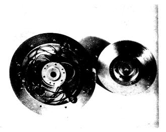
Figure 5 Interior of pressure transducer
