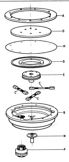
Figure 2 Exploded view of pressure transducer A. membrane clamping ring; B, transducer body; C. Cantilever; D, part of pressure plate; E, boss; M. sealing membrane; N, venting nozzle; P, plug
