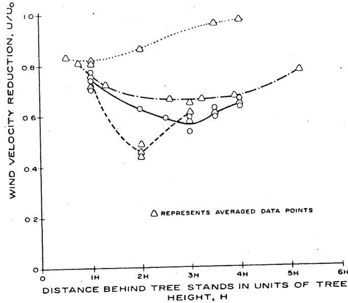
Fig.6. Sheltering effect for tree stands of different porosities in New Hampshire. Point line = low-porosity tree stand without leaves; dash-point line = low-porosity tree stand with leaves; full line = medium-porosity tree stand; dash line = low-porosity tree stand.
