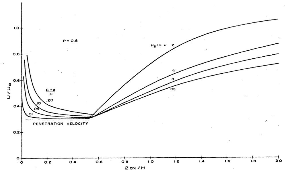
Fig.3. Effect of barrier geometry on theoretical wind velocity reduction.
