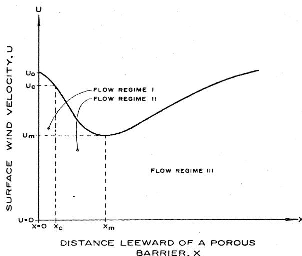
Fig. 1. The three flow regimes behind a porous barrier.
