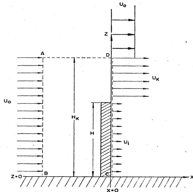
Fig.2. Idealized, frictionless wind flow through a uniformly porous barrier.
