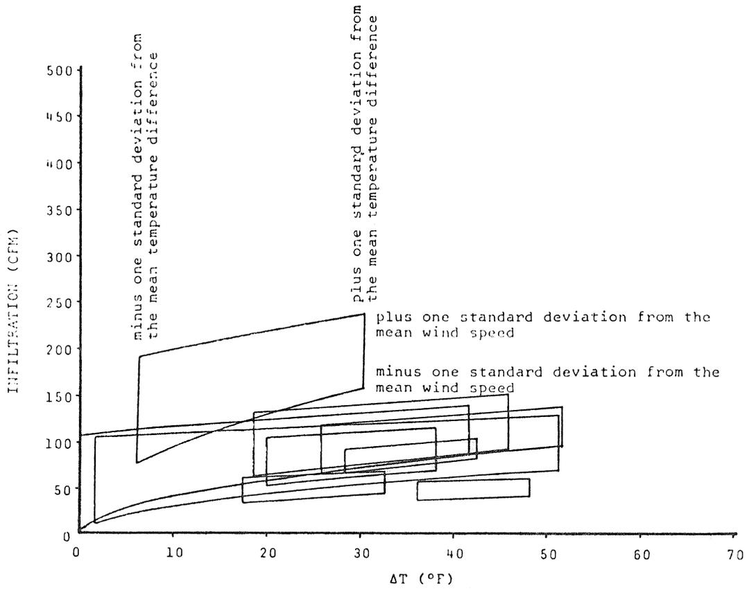
Fig. 3 Composite overlay of the measured data ranges
