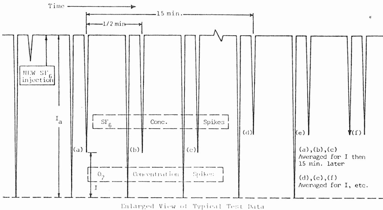
Fig. 2 Enlarged view of a typical chart record of air infiltration measurement
