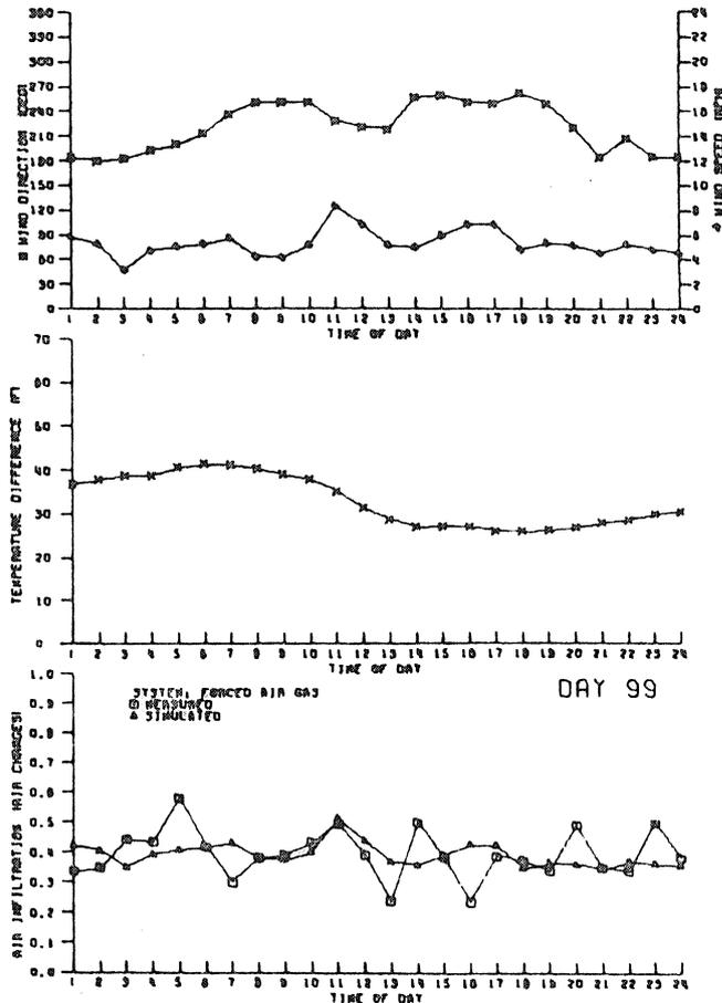
Fig. 7 Simulated vs measured air infiltration at site HSLG
