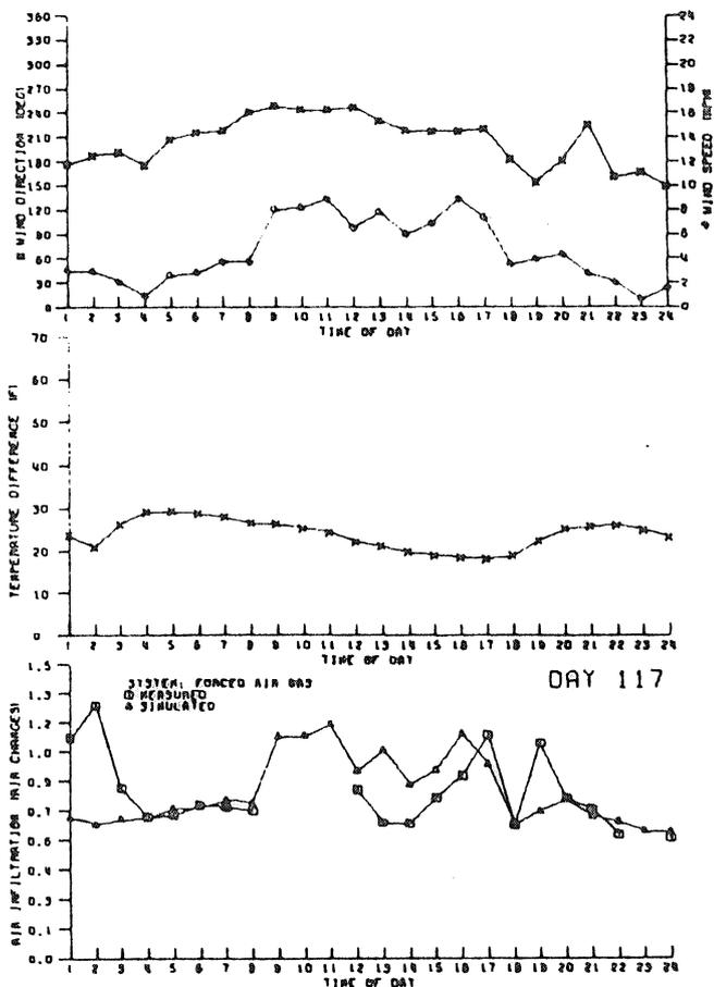
Fig. 6 Simulated vs measured air infiltration at site HTSG
