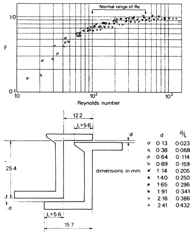
**Fig 2** Flow of air through window cracks
