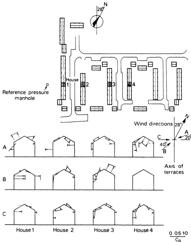
Fig 3 Effect of shelter on surface pressure coefficients
