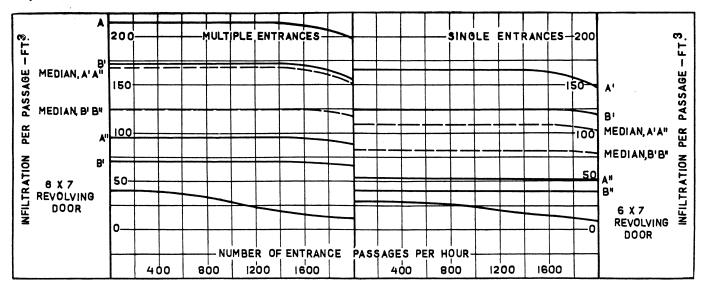
FIG. 4. COOLING LOAD LOSSES DUE TO DOOR FILTRATION IN MULTIPLE AND SINGLE ENTRANCE BUILDINGS.
