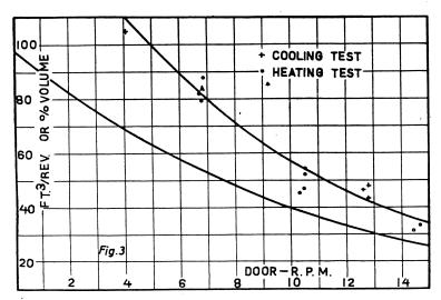
FIG. 3. DOOR FILTRATION IN TERMS OF DOOR REVOLUTIONS.
