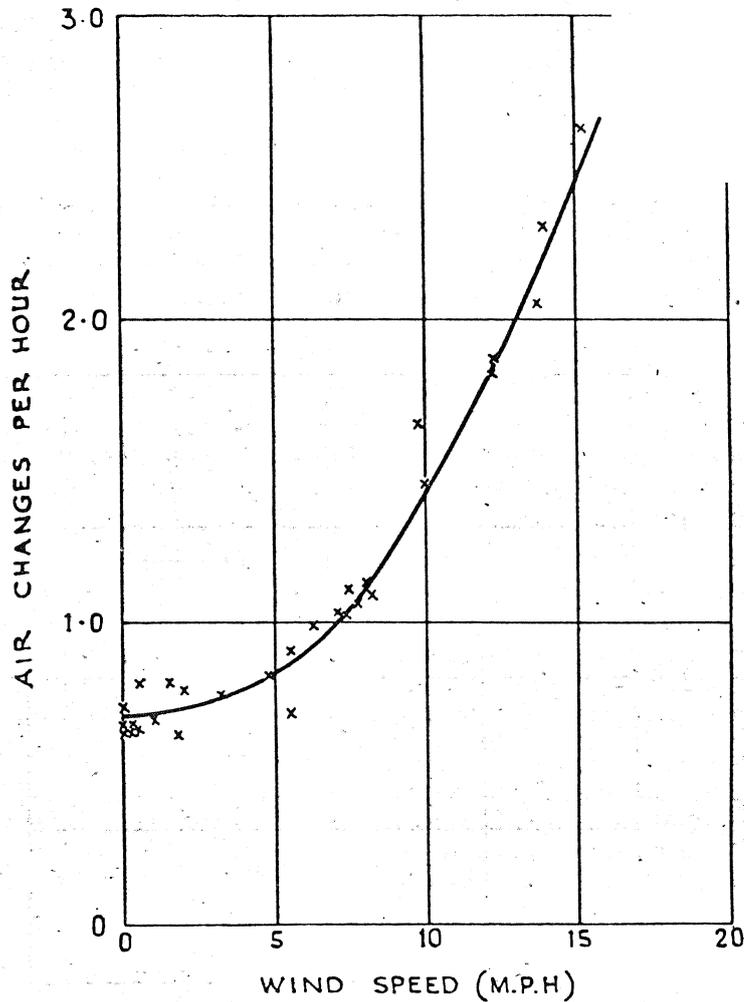
Fig. 5.—The Effect of Wind Speed on Air-Change Rate.
