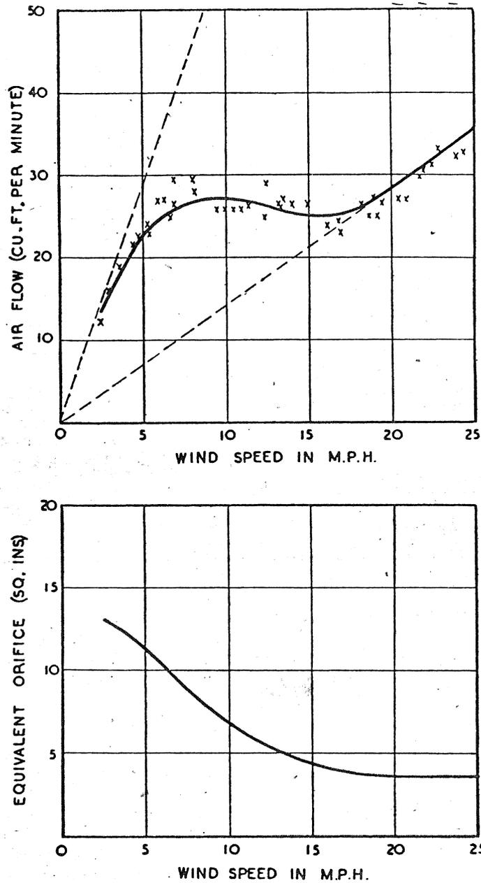
Fig. 2.—The Characteristics of Constant-Flow Ventilator.
