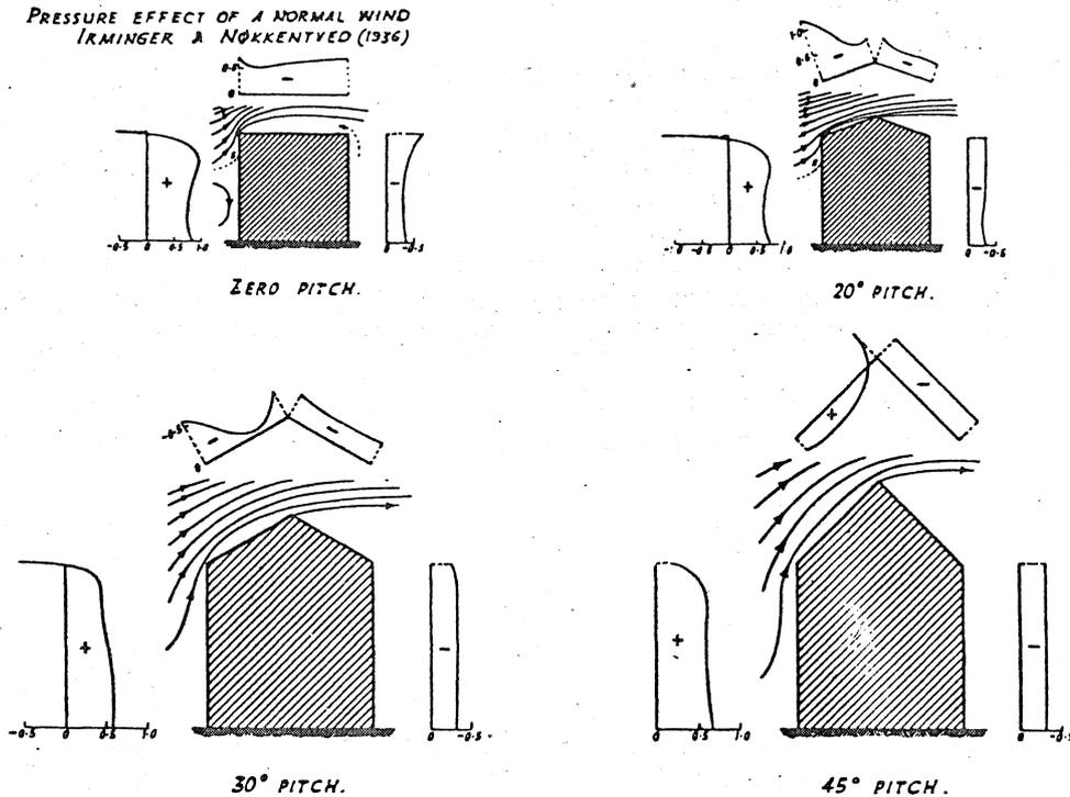
Fig. 1.—The Pressures Produced by a Wind Blowing Normal to a Building (Irmingier and Nøkkentved, 1936).
