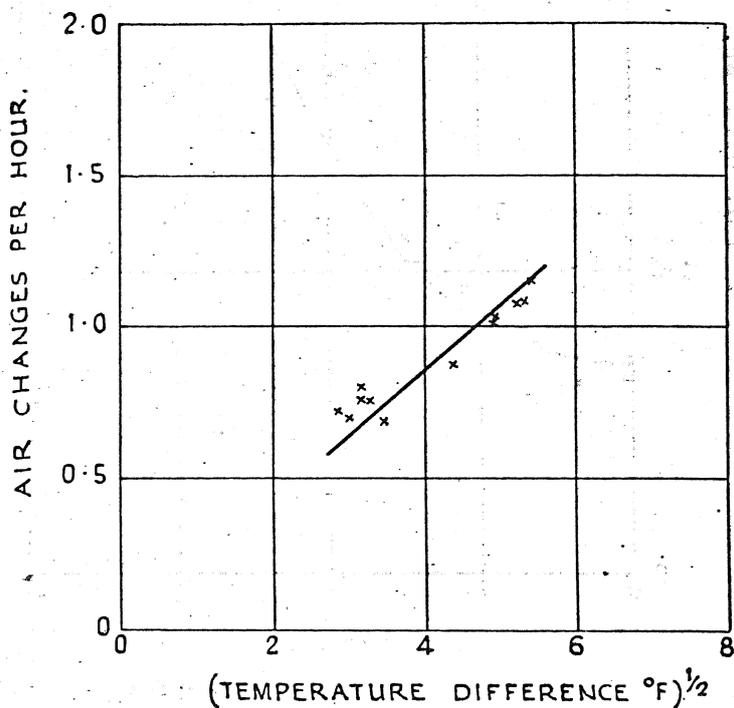
Fig. 4.—The Effect of Temperature Difference on Air-Change Rate at Low Wind Speeds.
