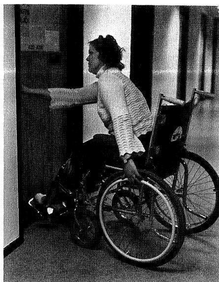
Checking the ability of a handicapped person to operate a weatherstripped door
