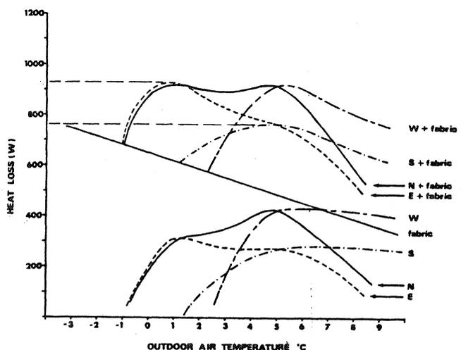
Fig. 4. Example of combined infiltration (wind effect) and wind fabric heat loss.
