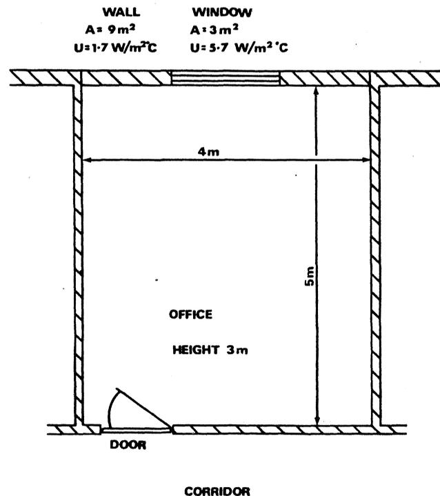
Fig. A2.1. Details of office construction used in example.
