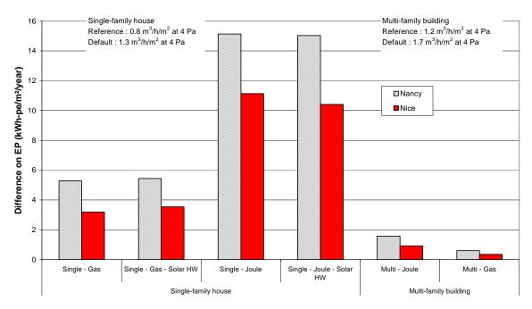
Figure 1: Examples of the energy impact (in kWh of primary energy) of envelope leakage in a single-family house and a multi-family building for the climates of Nancy and Nice (France), for extract-only relative humidity controlled ventilation systems.
