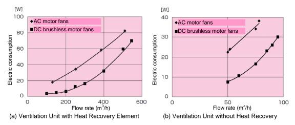
Figure 12 - Comparisons of Electric Consumption of Ventilation Equipment with AC and DC Fans
