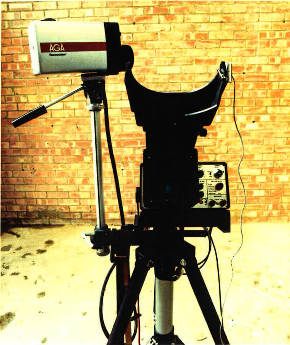
Figure 27 Application of thermography to wall tie detection
