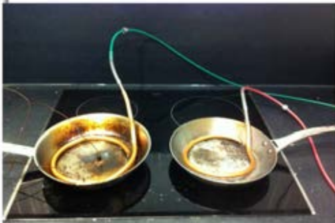
Figure 2. Induction method with CO 2 injection in two stainless steel 24 cm stir-fry-pans in the front locations, the left pan is equipped with temperature sensors. ¶
