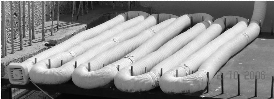
Preparation of the metallic base with the folded aluminium tube.
