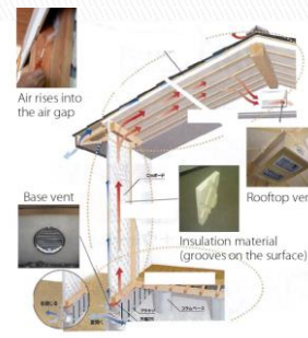
Double-skin system of room-side air gap
